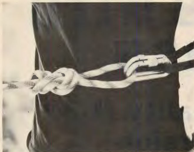
Figure-Eight Knot. Step 4: Pull figure-eight knot tight and clip into carabiners.
